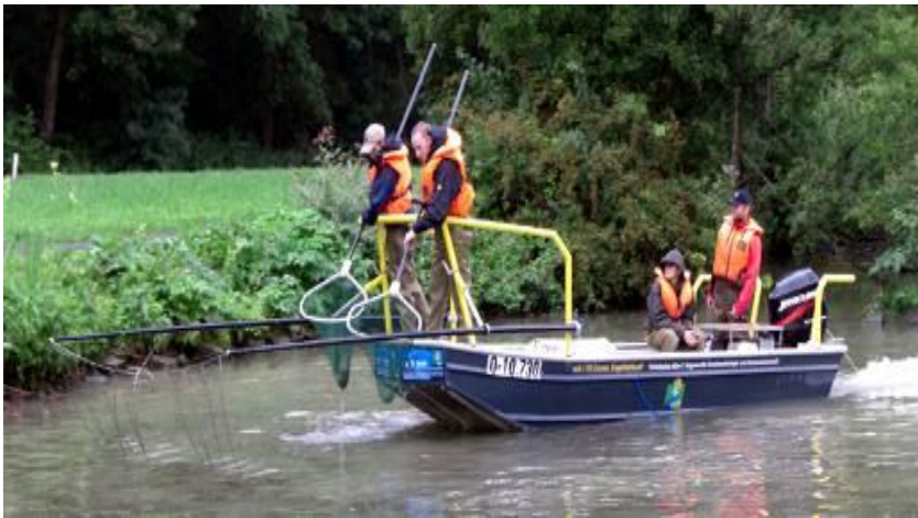
Photo 3. Power fishing device, for lakes, with compound anodes.
